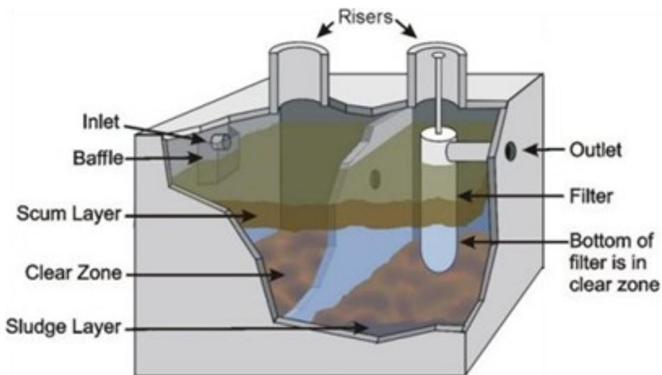
To ensure your effluent filter is working properly it should be inspected every year. Under normal conditions, your effluent filter will function for several years before cleaning is necessary.
